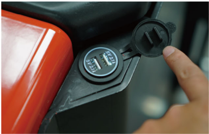
▴ Built in USB-connector USB-connector for charging of additional devices during warehouse operations.
