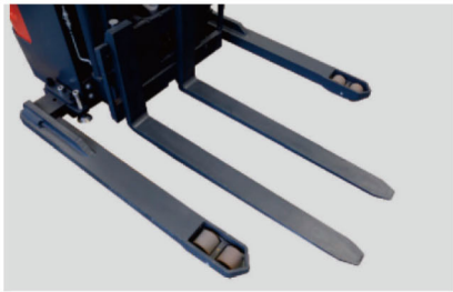
▴ Straddle leg Adjustable straddle leg design,suitable for diverse pallet sizes and more stability
