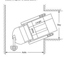
Aisle dimensions listed above assume the minimum bay width to be straddle OD plus 5" (2.5" on each either side of straddle leg). Straddle OD is the load width plus 10". Truck performance may vary due to application requirements' and changes in model design.
