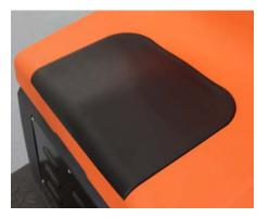
Operator Presence System (OPS) — When operator is not in seat, the scrubber will automatically stop.
