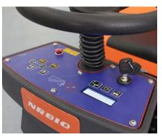
Integrated waterproof touch control panel with LCD for simple operation.
