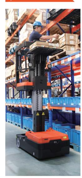
While platform is raising to its maximum height, the maximum available lift and drive speeds will go through three steps of speed settings according to the following lift height ranges for the platform: 0-19.7 inch, 19.7 - 59 inch, 59 - 118 inch to ensure the truck's stability and operator's safety.
